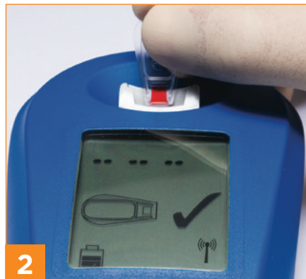
2 Insert the filled cuvette and press down gently
